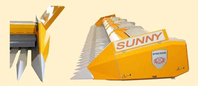
The new geometry of the sides allows it to penetrate the product without tearing it and eliminates the classic accumulation of product on external parts of the header. Unlike the competitors, Sunny presents a total protection that ensures three aspects that are primaries for us:
