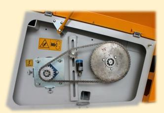
Flexible tensioners and constant lubrication minimize wear and friction on the chains; furthermore all the shafts are composed by hardened steel and supported by self-aligning bearings.
